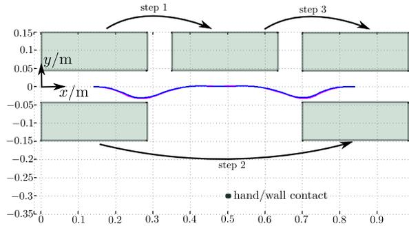
**Fig. 3** The resulting trajectory from the MPC scheme (8) for scenario 2 with hand support. In blue, the horizontal CoM trajectory produced after 2 steps of the algorithm (in 96 ms). In purple, the trajectory produced after 6 steps of the algorithm (in 412 ms). These trajectories are almost exactly the same, which shows that the convergence is fast.
