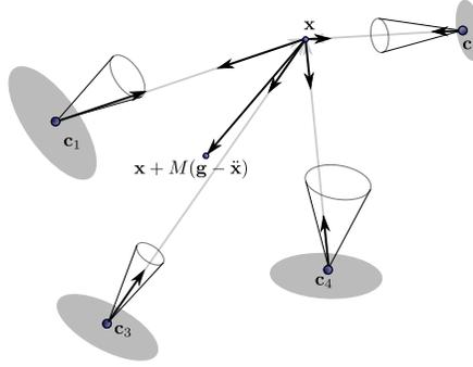
**Fig. 1** All the contact cones contain the direction towards the position of the robot CoM  $\mathbf{x}$ . Choosing the force of contact  $j$  equal to  $\alpha_j(\mathbf{c}_j - \mathbf{x})$ ,  $\alpha_j \geq 0$ , yields:  $M(\mathbf{g} - \ddot{\mathbf{x}}) = \sum_j \alpha_j(\mathbf{c}_j - \mathbf{x})$ ,  $\alpha_j \geq 0$ .
