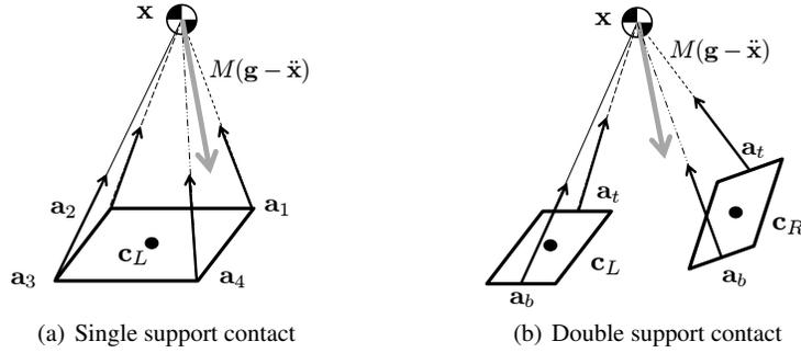
**Fig. 5** The constraints required to achieve dynamic balance for: (a) when one support is in contact with the environment  $\kappa_L = 1, \kappa_R = 0$  and (b) when two supports are in contact  $\kappa_L = 1, \kappa_R = 1$ .
