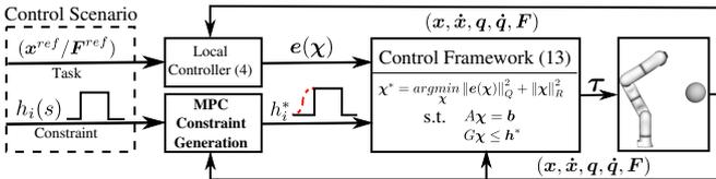
Fig. 6: Block diagram of the control framework.
