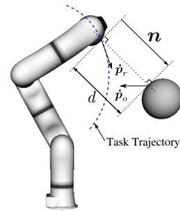
Fig. 1: Description of the obstacle avoidance constraint.
