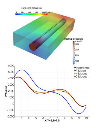
Fig. 2: On the left panel, we have a snapshot of the reference solution for t = 0.006. The tube is the domain  $\Omega_1$  where we solve the Stokes equations. On the right panel pressure  $p_1$  at the black line of the left panel has been displayed for different choices of the offline basis' dimension that are compared to the reference solution.
