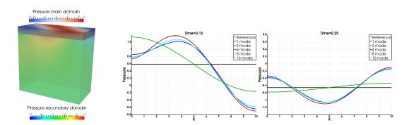
Fig. 1: A snapshot of the reference solution for t = 0.15 (left panel). Pressure p at the interface  $\Gamma$  (first test case) along the line y = 2.5 for two different time instants (center and right panel). Finite elements results are compared with the reduced approach for different numbers of modal functions.
