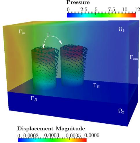
Fig. 4: Solution of the complete problem at time  $t = 0.00325102$ . The color scale on the cylinders and on the basement represent the displacement, while the fluid domain is colored by the value of the pressure and transparent.
