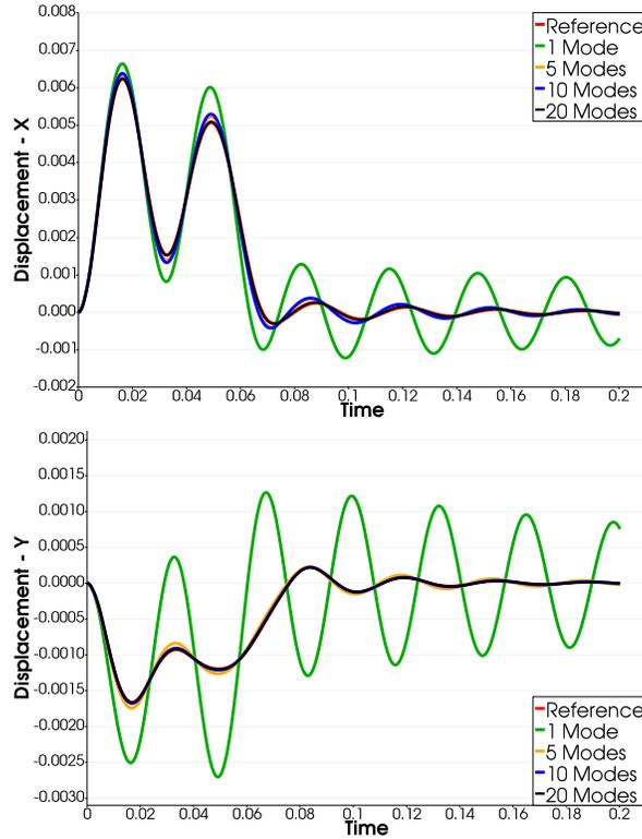
Fig. 6: The displacement of the center point on the top of the first cylinder:  $x$ -component on the left and  $y$ -component on the right. The reduced approach is compared with the reference, finite-element, solution by varying the number of modes in  $\{1, 5, 10, 20\}$ .
